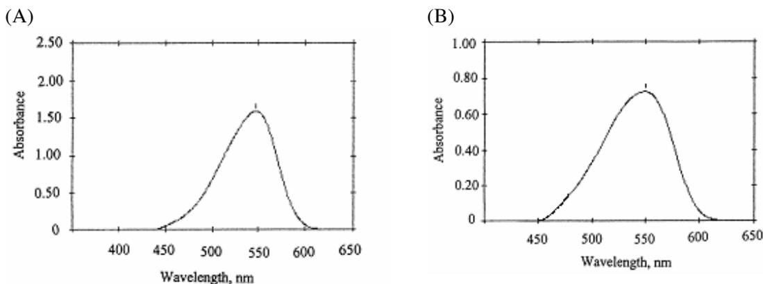
**Figure 1.** Absorption spectra of the reaction products of DAP (A) and MET (B) with p-DAC.
